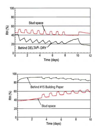
As can be seen, the moisture conditions of the two walls are very different even though the laboratory conditions are equivalent. Behind the DELTA<sup>®</sup>-DRY, the relative humidity drops over the test period as the solar heating dries the sheathing board (OSB). Each time the heating lamp is on, the relative humidity in the stud space increases, but over the duration of the test, the relative humidity in the stud space is dropping. This indicates that drying is occurring.
