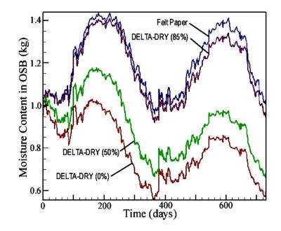
although the disparity between the performance of the DELTA<sup>®</sup>-DRY wall and the sheathing paper wall was naturally not as great in warm and hot climates as in cold to mixed climates.
