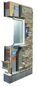
designed to be installed on the exterior sheathing board (OSB) as a substitute for conventional sheathing membranes (i.e. building paper). It may also be installed over breather type sheathing membranes or building
